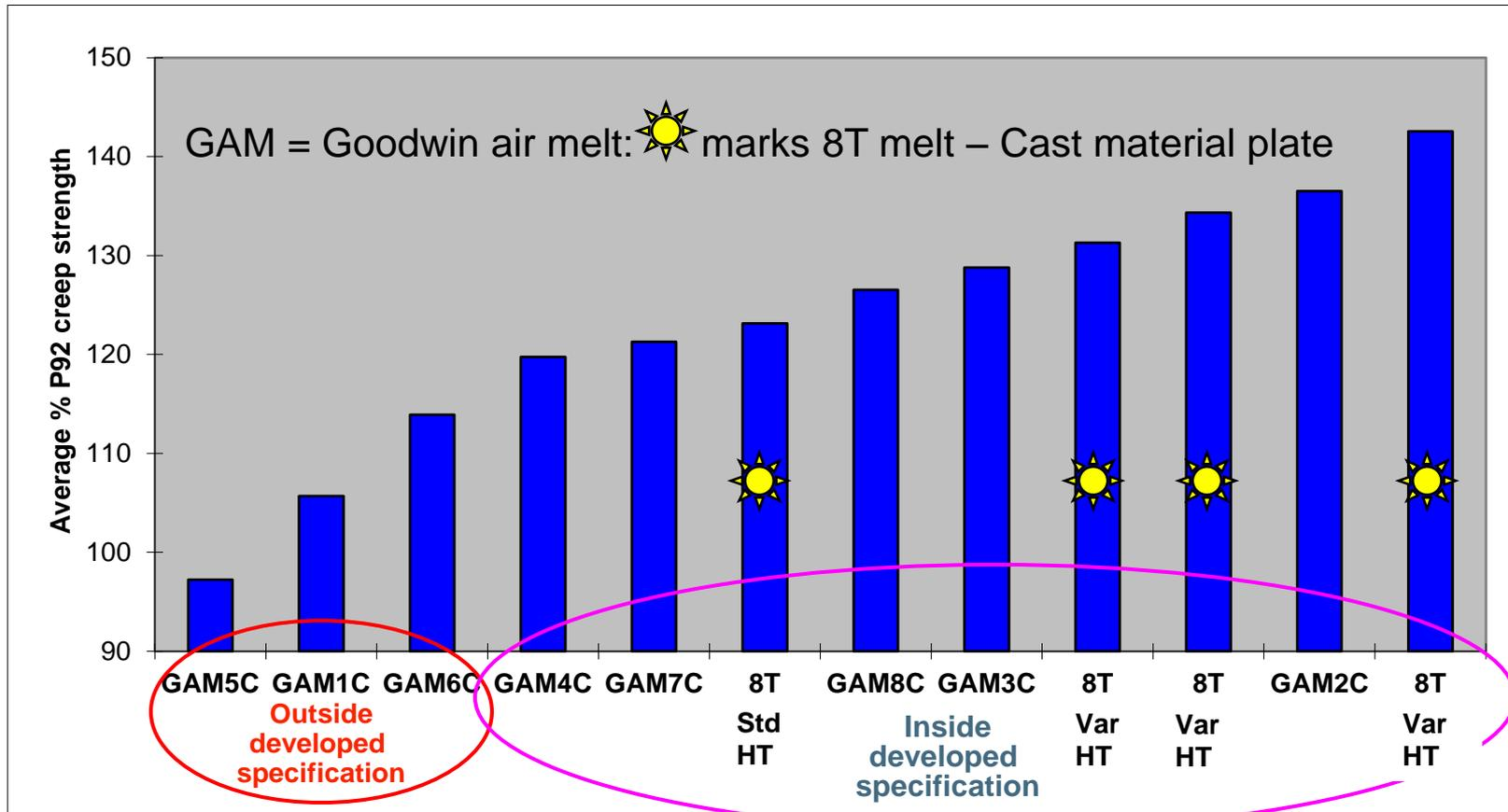
Within wide specification range, MARBN showed 20-40% greater creep strength than P92, indicating  $\approx 25^\circ\text{C}$  higher capability, saving  $\approx 2\%$  in fuel costs and  $\text{CO}_2$  (much more vs. older plant)
